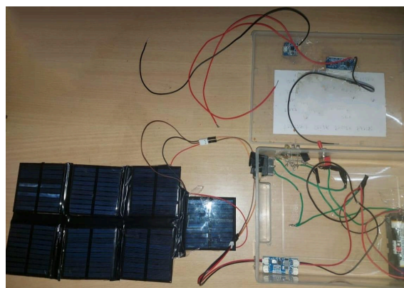
Fig1. Solar power bank internal circuitry
