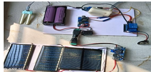
Figure:4 Charging of battery using solar panel
