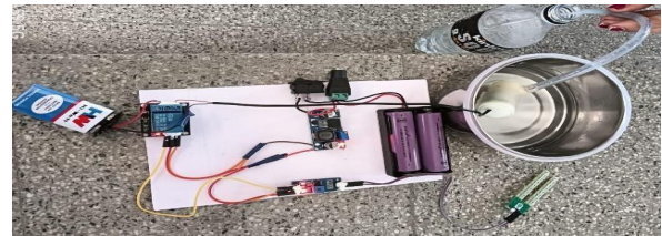
Figure:4 Water pump is on when moisture sensor is in dry
