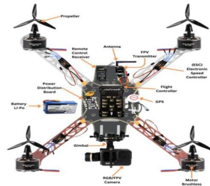
Figure: 1 Quadcopter Parts
