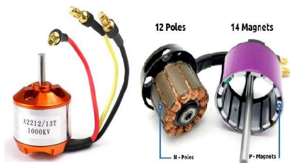
Figure 6: BLDC Motor construction [10]
