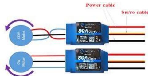
Figure 5: ESC CW and CCW motor connection
