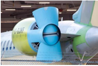
Figure 22 Aircraft Target type thrust reverser in deployed position
