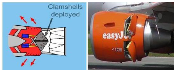
Figure 11 Clamshell reverse thrust design.
