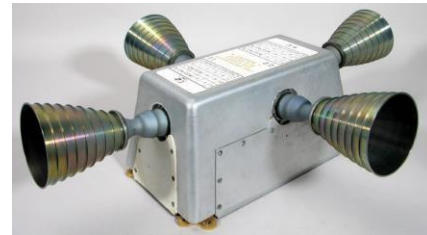
Figure 4 Apollo Reaction Control Systems (RCS)
