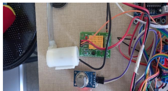
Fig 16: Gas sensor and gas cylinder with a pipe connected
