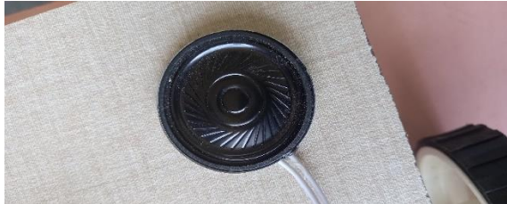
Fig 18: Miniature speaker to play recorded voice
