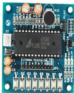
Fig 7: APR 33A3 voice recording module
