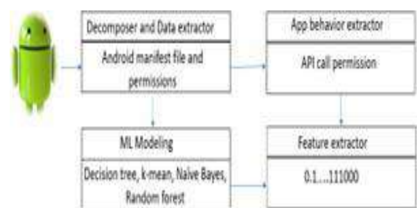
Fig 3: The proposed permission and API call feature-based malware detection framework.
