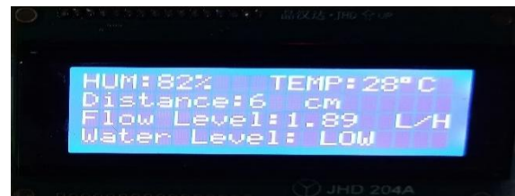
Fig 3: LCD displaying data
