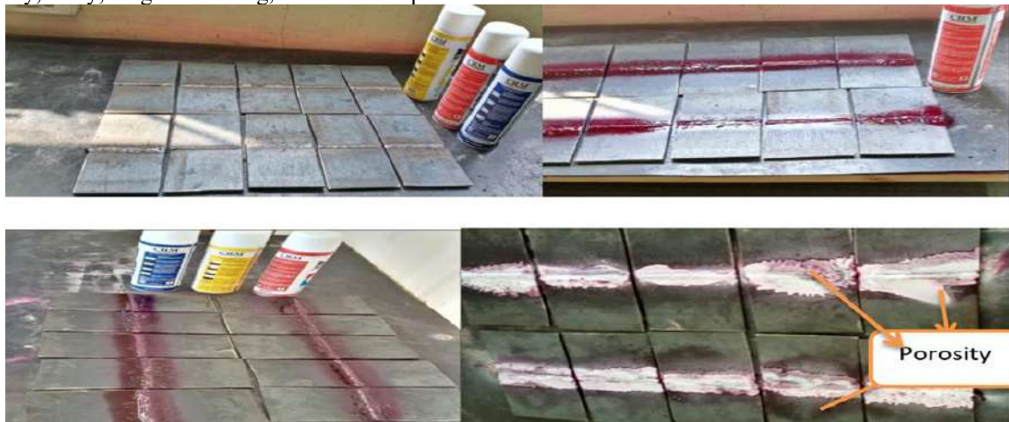
Figure 3: Welded specimens after LPT modified setting, source: (Metal Industry Development Institute)
