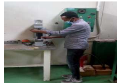
Figure 6 Vickers's hardness testing machine and hardness test specimen
