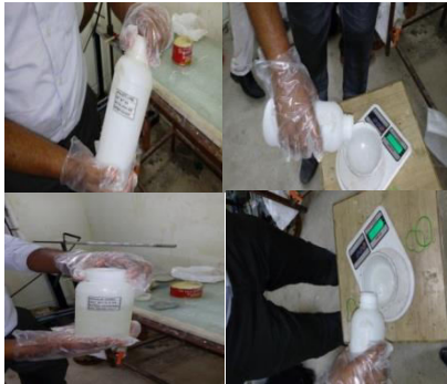
Fig.8 Resin and hardener preparation
