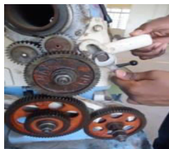
Fig 10 Change over the lead screw direction
