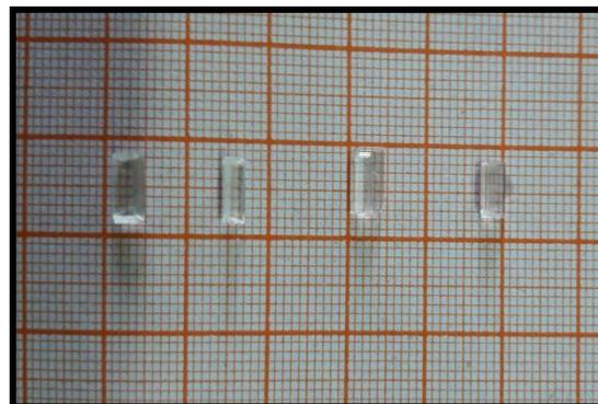
**Figure 3.1** As-grown crystals of LTTF
