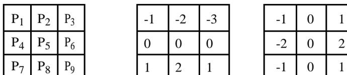
Fig.3.Example Block for sobel mask
