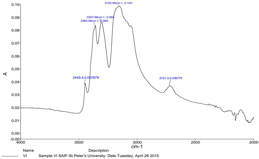
**Fig 3.3 FT-IR spectra of MgSO<sub>4</sub> doped ZTS crystal**
