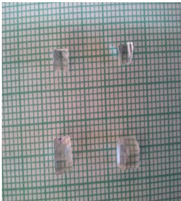
**Fig.3.1 Photograph of grown MgSO<sub>4</sub> doped ZTS crystal**
