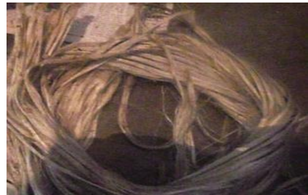
Figure 2.2 Extracted Fibre From The Aerial Roots Of The Banyan Tree
