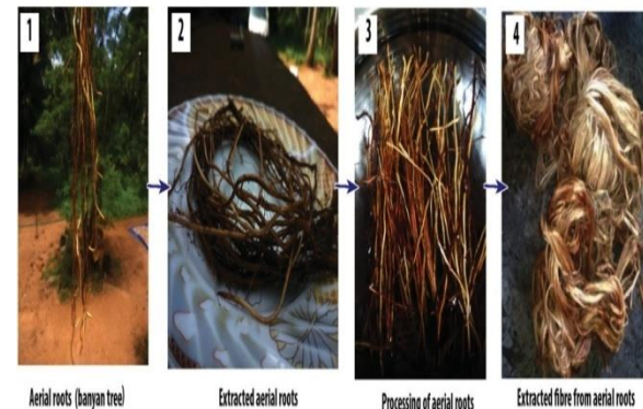
Figure 2.1 Process Of Extraction Of Fibre From The Banyan Tree Aerial Roots
